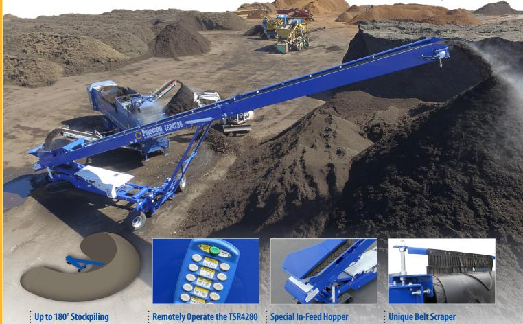
With up to 180° of rotation, you can stack even larger piles. The radial movement allows greater volume and control where you want to put your product.
